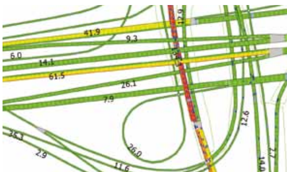
(Left) The Aimsun traffic model for the Pan Am games area comprises a larger mesoscopic-level area with some pockets of microscopic modeling
