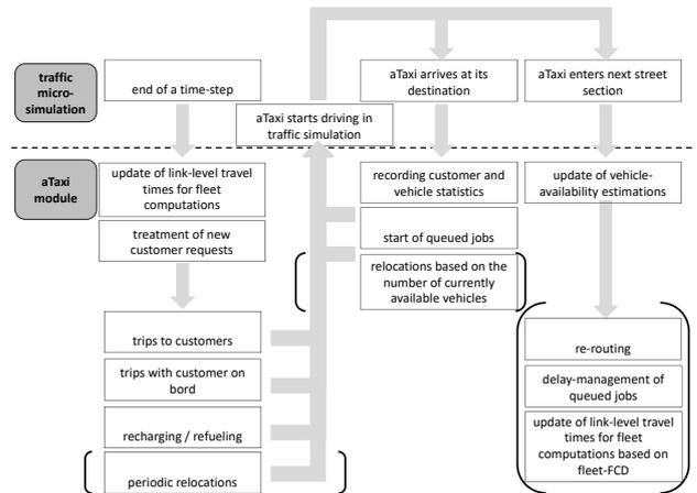
(b) Interface of the aTaxi module and the traffic microsimulation. Actions in brackets are not included in this work.
